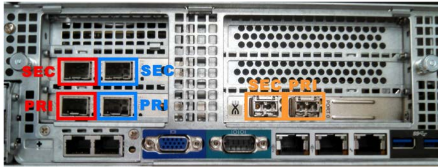
Figure 1. Example HCP G10 configured with 10G SFP+ ports for both front- and back-end connections with an additional pair of bonded Ethernet ports.
